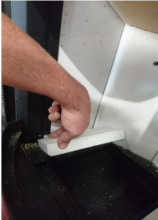
*Remove grate and base fire bricks.*
