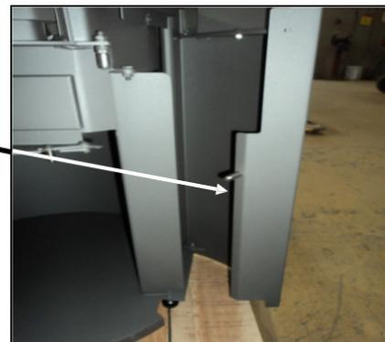
In this picture, the foot is displayed with which you can adjust the stove so that the automatic locking mechanism can function properly.
