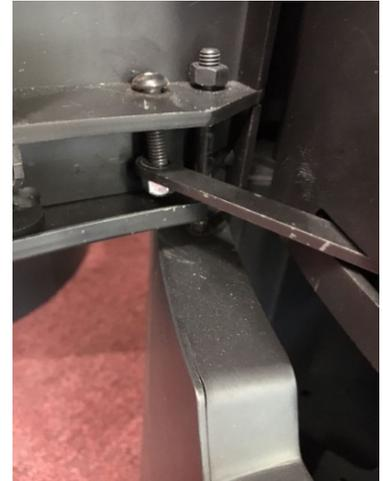
When the stove is out keep both regulators closed, in order for cold air not to be able to circulate throughout the chimney. However, it can be advantageous to open the air controls awhile before lighting the stove to allow warmer air to begin going up the chimney.
