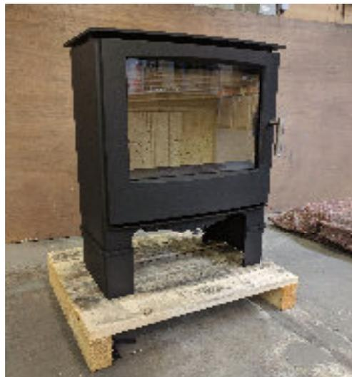
Right the stove and see if the legs are in the correct position; they should be inline with the front legs of the Woodand / Loxton and have an even overhang where the legs meet the stove body. If not then loosen one leg at a time and adjust until satisfied.
