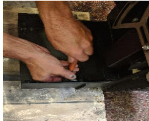
Position the Logstore legs and use the levelling feet to secure them to the body of the stove. Use a spanner or a socket wrench to fully tighten.
