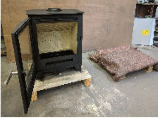
Remove the internal components of the stove and fill the chamber with material to prevent the bricks from falling. Additionally, prepare a soft elevated surface.
