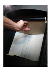
Now lower the throat plate baffle to remove.
