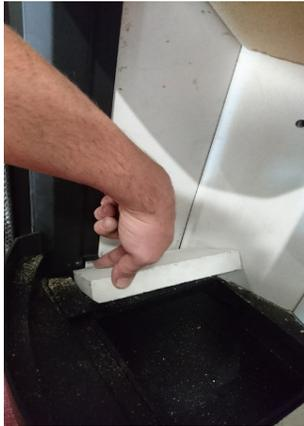
*Remove grate and base fire bricks.*
