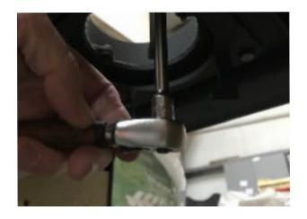
4) Remove Catalyst holder by unbolting 4 M8 bolts using a 13mm Socket
