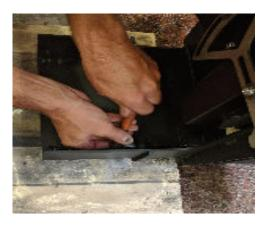
Position the Logstore legs and use the levelling feet to secure them to the body of the stove. Use a spanner or a socket wrench to fully tighten.
