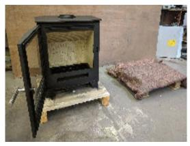
Remove the internal components of the stove and fill the chamber with material to prevent the bricks from falling. Additionally, prepare a soft elevated surface.
