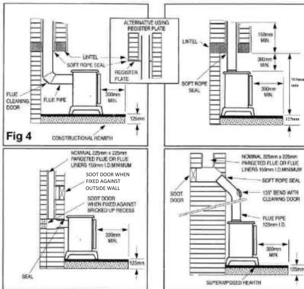
If there is no existing chimney then either a prefabricated block chimney in accordance with Building Regulations Approved Document J or a twin walled insulated stainless steel flue to BS 4543 can be used. These chimneys must be fitted in accordance with the manufacturer's instructions and Building Regulations.
